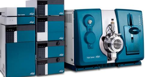
ExionLC AD coupled to a Sciex QTRAP 6500<sup>+</sup> mass spectrometer (Sciex, Concord, Ontario, Canada). **Target analytes:** -5 Pesticides Perfluoroalkyl -5 substances (PFASs)
