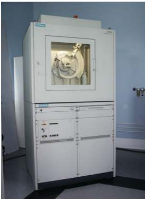
Figura 3.9 Difractómetro, Siemens D5000 diffractometer with Cu K \alpha radiation. [35]
