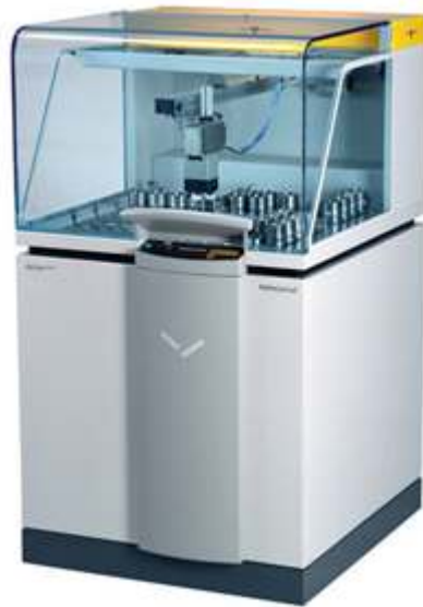
Figura 3.7 Espectrómetro, Panalytical Axios wavelength dispersive (4 kW). [28]
