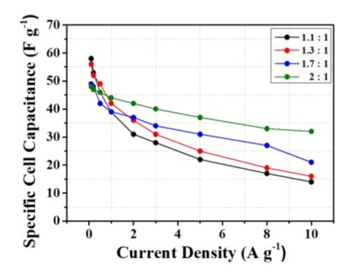
**Figure S2.** The specific cell capacitance evolution of the different LIC devices assembled using the labeled negative to positive mass ratios.
