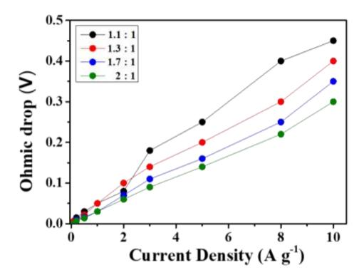
**Figure S1.** Comparative ohmic drop values with respect to different current densities for the different LIC devices assembled using the indicated positive to negative mass balances.
