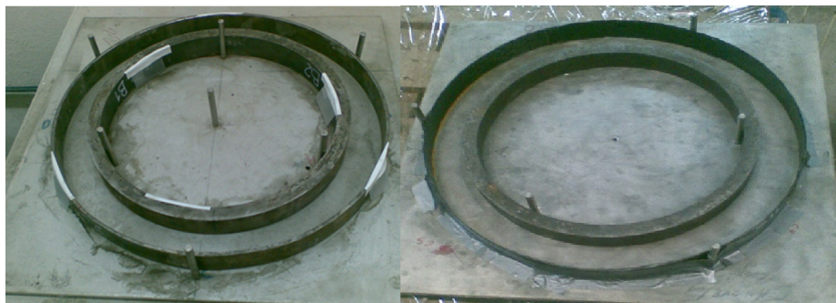
Fig. 11. Double-ring test device with outer steel jacket (left) and CFRP jacket (right)-
