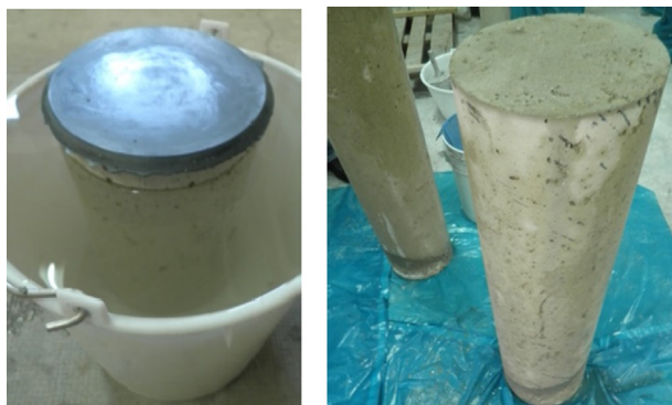
Fig. 4. Moistened specimens-left (immersion) and reinforced concrete columns-right (irrigation).
