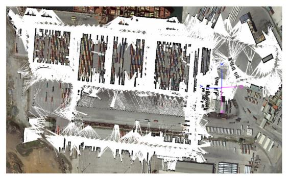
**Figure 11.** The map is overlaid onto a georeferenced image using the optimized EN-to-SLAM frame transformation  $(X,Y,\theta)=(4.01m,3.42m,3.177rad)$  with an EN origin at (1at,lon)=(40.638972,22.907978). Notice that the image and the map correspond to different days and hence some of the mapped features do not match.
