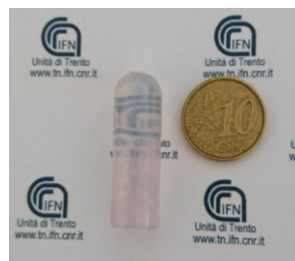
Figure 2. Photo of the fabricated 95SiO 2 -5SnO 2 :0.5Er 3+ big pillar (1 cm diameter and 3.3 cm length) obtained after heat-treatment at 900 °C for 100h 11 .
