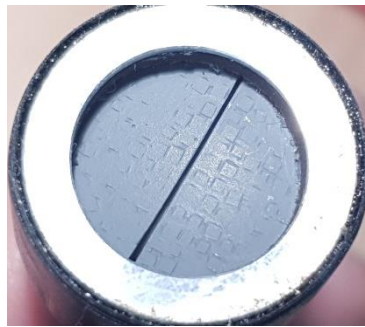
Figure 2. Focused 0.9 MHz 15 mm diameter dual piezoelement transducer used for transmission.
