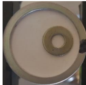
Figure 9. Steel spacer as artificial defect placed on probe's surface.
