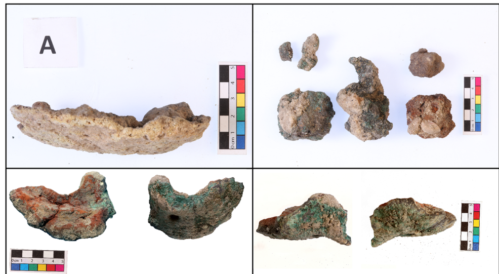
Fig. 4 Some specimens recovered from Emporion representing the typical finds: Fe slag cake (top left), Cu-based slags (top right) and different views of the tuyère 1311;B4/5 (bottom)
