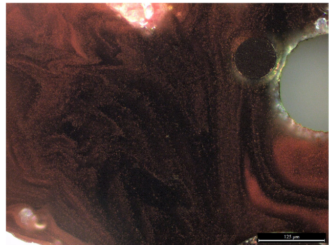
Fig. 8 OM micrograph of sample 11146-2 under reflected XPL light showing fine exsolution of cuprite within the slag. Note the metallic copper prill (black) next to a large round pore (top right). (Scale = 125 μm)
