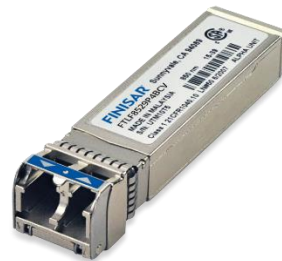
Fig. 1.17. Right: types of optical mechanical connectors. Left: Example of an active transceiver part SFP+ connector from Finisar Corporation with a LC mechanical connector socket.
