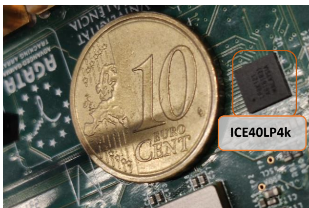
Fig. 5.6. Size of the ICE40LP4k in relation to a 10 cent coin
