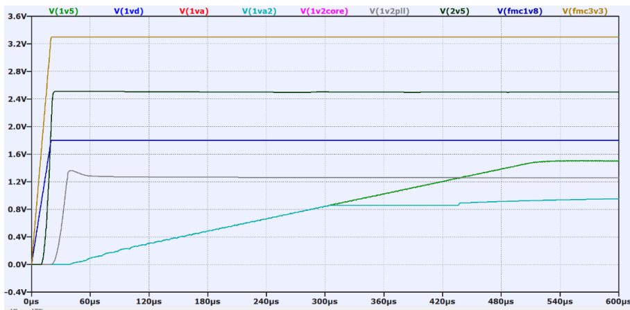
Fig. 5.16. The IDM power simulation schematic and plot, the first 7 are the generated supplies, the resting are from taken from the FMC connector.
