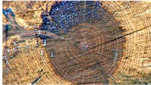
Fig. 2 Detail of the heartwood of the Canary pine or Pinus Canariensis , a protected tree species in the archipelago. Its wood shows a sharp contrast between the sapwood, or outer part, and the heartwood, or inner part. The first is soft and yellowish-white in colour; the inside, the tea , is very resinous and has a reddish colour. It takes at least 30 years for the tree to start forming tea . The tea is practically incorruptible and solid, and has always been highly prized in construction. Source: authors
