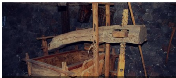
Fig. 5 Winepress made of tea . Winepresses consisted on a large beam and a spindle. The wine was bundled together with a tight rope forming the so-called ' queso ' (cheese) before pressing the wine. The wine then fermented with stems and skins in a basin or ' lagarillo ' before being transferred to the tea casks, or it could also ferment within the tea casks immediately after crushing the grapes. Source: authors
