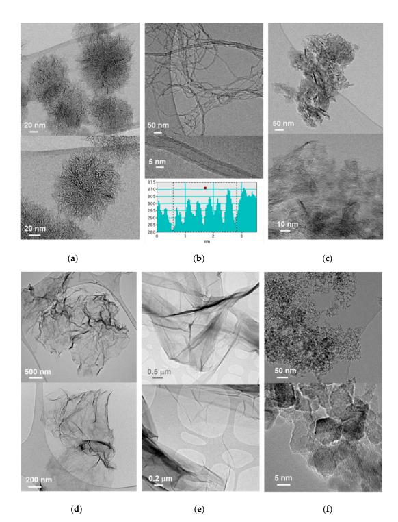
**Figure 1.** TEM micrographs of the tested carbon nanomaterials: (**a**) CNH, (**b**) CNT, (**c**) CNP, (**d**) RGO, (**e**) GO and (**f**) ND. Inset in (**b**) shows image analysis of a MWCNT with six concentric nanotubes.
