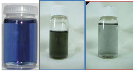
Figure 1: Polyaniline Composite Dispersions: a) Emeraldine base with CNTs, b) Emeraldine Salt with reduced graphene oxide (RGO), c) Emeraldine Base with graphene oxide (GO).
