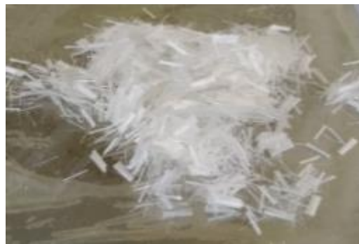
Figure 3.12. General appearance of PVA fibres used in this work
