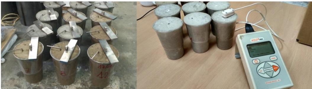
388 Figure 1. Mortar samples curing with the pilot pins inserted inside (left) and thermal conductivity
