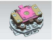
Figure 1. 3D model of the design of hightemperature part of exchangeable sample holder.
