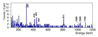
FIG. 3. Sum of projections from a  $\gamma$ - $\gamma$  coincidence matrix from the RIBF83 experiment. Gates were placed on the eight strongest transitions and the resulting spectra were added together.
