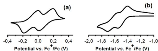
**Figure 1.** Cyclic voltammograms of **1** (a) and **2** (b) recorded at room temperature under Ar atmosphere ( $10^{-4}$  M/0.03 M TBA-PF<sub>6</sub>/o-DCB).
