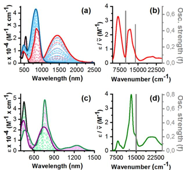
**Figure 2.** Electrochemically obtained ( $10^{-4}$  M/0.03M TBA-PF<sub>6</sub>/o-DCB) UV-Vis-NIR absorption spectra during oxidation of **1**: (a) neutral species, black solid line; radical cation, red solid line; dication, blue solid line, and reduction of **2**: (c), neutral species, black solid line; radical anion, green solid
