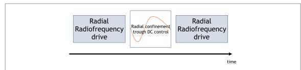
$\textbf{Figure 5.} \ \ \text{Experimental control sequence.} \ \ \text{The radial radio frequency drive is switched off during the application of the shortcut to adiabaticity protocol on the DC electrodes, the shortcut changes the radial confinement.}$
