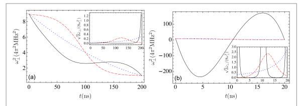
**Figure 3.** Radial confinement squared for a linear ramp (blue dotted line), smooth ramp (red dashed line) and the shortcut to adiabaticity (black solid line), with (a) parameters chosen to avoid negative  $\omega^2$  and (b) allowing negative  $\omega^2$  for the shortcut. Here,  $\omega_0/(2\pi)=3$  MHz and  $\omega_f/(2\pi)=1$  MHz. Inset: Adiabaticity parameter  $\sqrt{2}\,\dot{\omega}/(8\omega^2)$  for the three cases.
