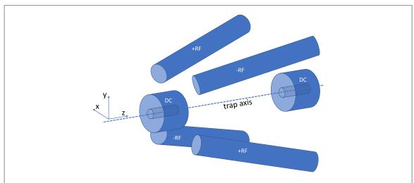
**Figure 1.** Tapered ion trap. The tapered electrodes are supplied symmetrically with radiofrequency voltage for the radial confinement. Endcaps are used to supply axial confinement with DC voltages. During shortcut to adiabaticity protocol the radiofrequency is switched off and the voltage on the endcaps is used to realize the axial confinement or anti-confinement, respectively. Due to the short duration stable trapping conditions can be maintained.
