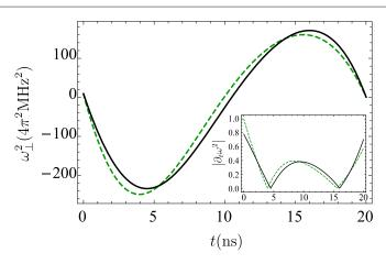
**Figure 2.** Radial confinement  $\omega^2$  as a function of time for two different designs of the shortcut. (Green dashed line) Standard 6-order polynomial fulfilling the frictionless conditions (8). (Black solid line) Improved design with extra-coefficients to control the value of  $\max |\partial_t(\omega^2)|$ . The inset shows  $|\partial_t\omega^2(t)|/|\partial_t\omega^2(0)|$  for both designs. Here,  $\omega_0/(2\pi)=3$  MHz and  $\omega_f/(2\pi)=1$  MHz.
