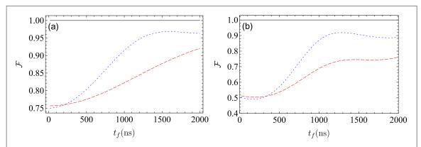
**Figure 4.** Fidelity  $\mathcal{F}(\hat{p}(t_f), \hat{p}_{\text{target}})$  as a function of the expansion time  $t_f$  for three different protocols, shortcut (black solid line), linear ramp (blue dotted line), and smooth ramp (red dashed line). In (a) the initial state corresponds to a thermal state with temperature of 2 mK. In (b) the initial state is a coherent state with a photon number  $\alpha_0 = 1 + i$ . Parameters as in figure 3.
