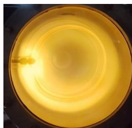
Discharge chamber, detector of millimetric radiation and focusing set-up in the Observatorio Astronómico of Yebes to study the rotational emissions of radicals and molecules generated in cold plasmas.
