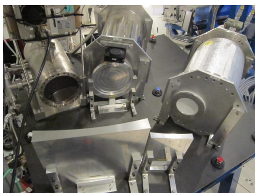
Discharge chamber, detector of millimetric radiation and focusing set-up in the Observatorio Astronómico of Yebes to study the rotational emissions of radicals and molecules generated in cold plasmas.
