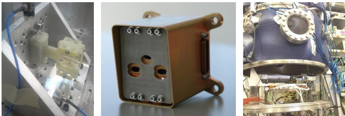
Figure A11: Different validation models of MEDA sensors. From left to right. ATS (Ambient Temperature Sensor), TIRS (Thermal InfraRed Sensor) y WS (Wind Sensor).
