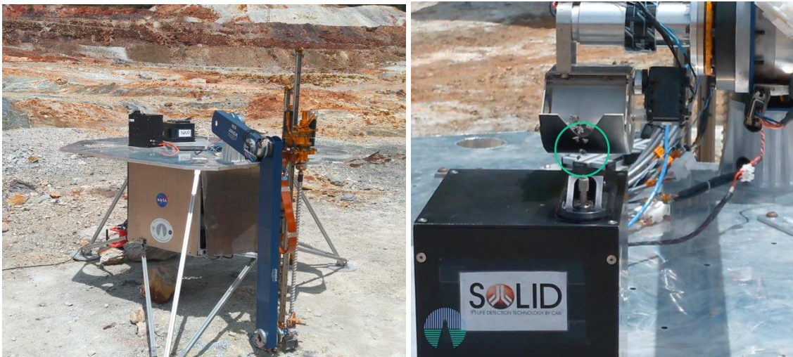
Figure ME17: LMAP campaign in rio Tinto. (left) NASA Phoenix mockup equipped with a robotic drill, arm, and scoop to collect a sample from the subsurface and load SOLID for processing and searching for microbial markers with LDChip. (right) The scoop delivering a small amount of material to the SOLID sample extraction cell.
