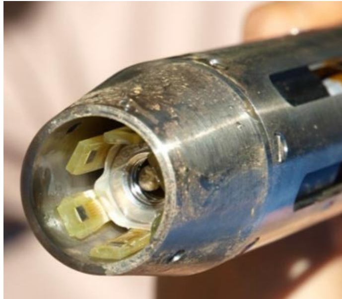
Figure A18: Prototype of the geo-biological characterization system of the subsoil during final field trials
