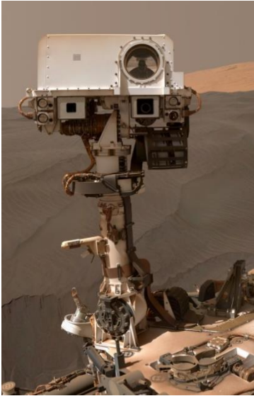
Figure A15: Photo of the boom 2 and REMS UV sensor taken by one of the Curiosity cameras in a landscape of Martian dunes. In boom 2 you can see the air temperature sensor, the humidity sensor, the wind sensor.
