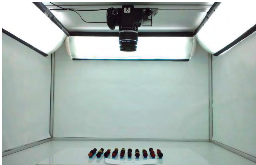
Figure 16: Inspection chamber for berry image acquisition. The berries were placed in a plate for proper image acquisition, the camera and the illumination were positioned in top of the chamber.
