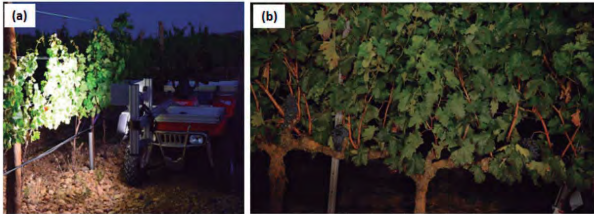
Figure 2. (a) On-the go Image acquisition with the multi-sensor mobile platform; (b) Image acquired with artificial illumination in which, due to appropriate illumination and camera parametrization, the vines under evaluation are discernible from the darkened background.
