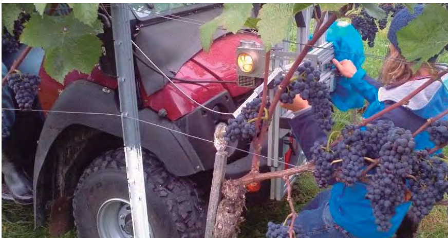
Figure 10: Adjustment of an ATV mounted experimental spectrometer for non-destructive assessment of berry composition.
