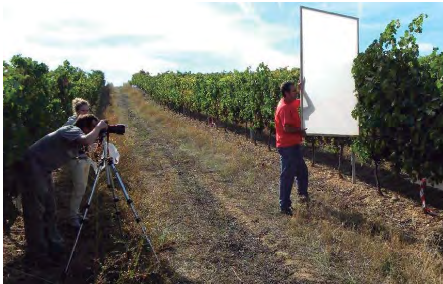
Figure 17: Manual vine imager acquisition using a tripod mounted digital camera, controlled background and semi-controlled illumination (use of a diffuser to avoid direct-sunlight).
