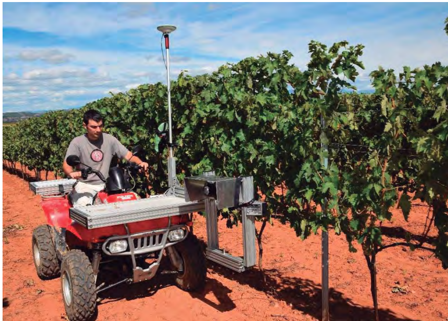
Figure 19: Modified ATV for on-the-go RGB image capture. The vehicle is equipped with automatic triggering, camera and GNSS receiver.
