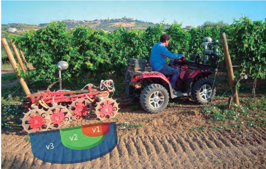
Figure 13: A resistivity soil sensor for on-the-go operation in a vineyard located in La Rioja appellation. The four rolling electrodes enabled measurements on approximately 0.5, 1 and 2 m depths.
