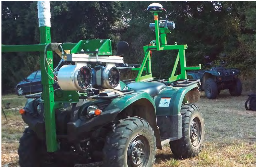
Figure 8: Multiplex sensor (Force A) mounted on an ATV.
