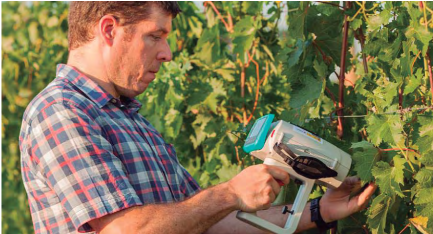
Figure 9: Manually operated punctual radiometer.
