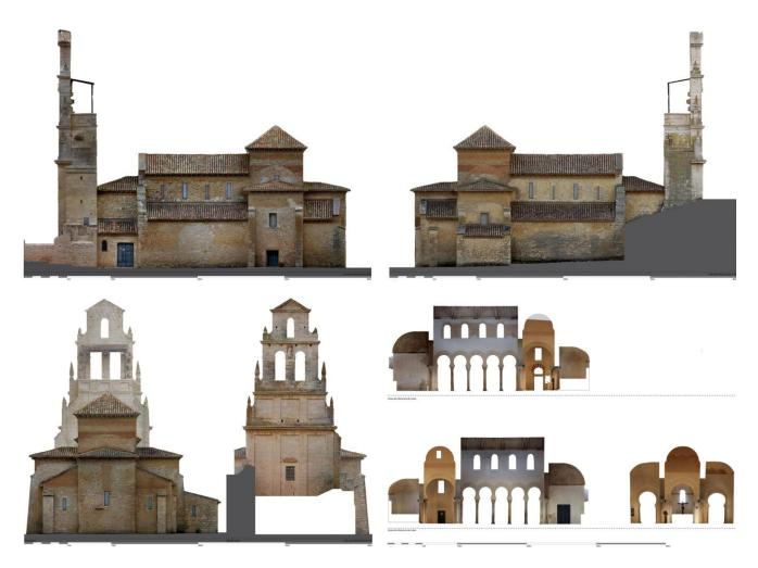
Fig. 2: Orthoimages of the external façades and main inner walls
