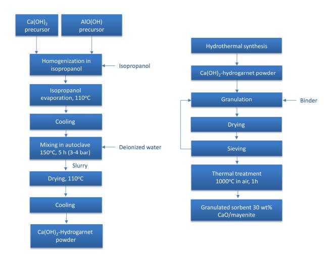
Figure S2: Scheme for preparation of sorbent including hydrothermal synthesis (left) and granulation/calcination (right)
