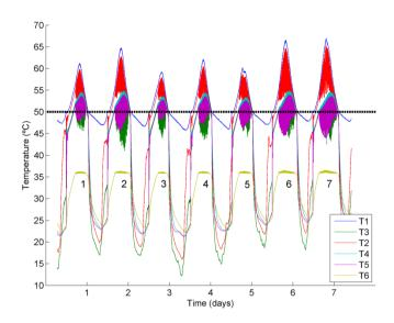
Figure 12 Experiment 1 temperatures on the solar circuit and inside the incubator. In the last two days of the experiment, there was enough heat accumulated to extend the use of hot water
