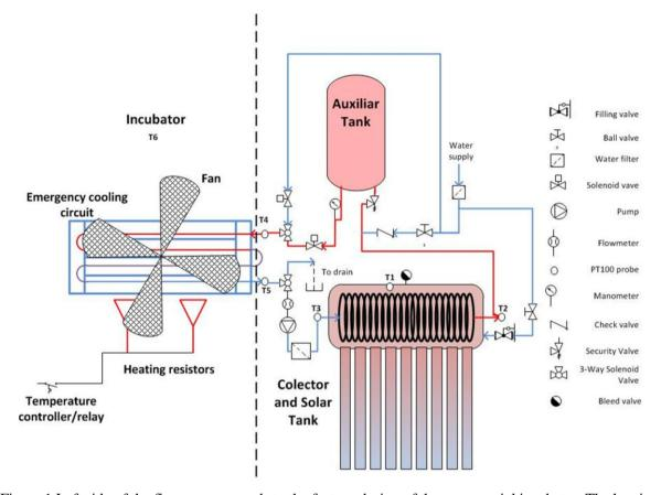
Figure 1 Left side of the figure corresponds to the factory design of the commercial incubator. The heating resistors have a total power of 1.7 kW. The right side of the figure shows the hydraulic diagram of the solar heating system and the coupling to the commercial incubator.
