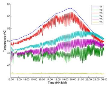
Figure 3 Temperature evolution during the solar contribution period for Experiment 1. Temperature monitoring at five locations of the solar circuit and the incubator
