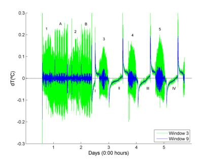
Figure 8 Representation of the smoothed derivative of the temperature inside the incubator using the Savitzky-Golay algorithm for windows of three and nine elements
