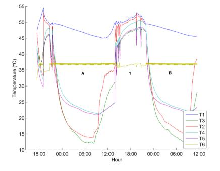
Figure 10 Experiment 3 temperatures. 'A' and 'B' are periods with electrical heating. During the 'A' period, there is solar heating.
