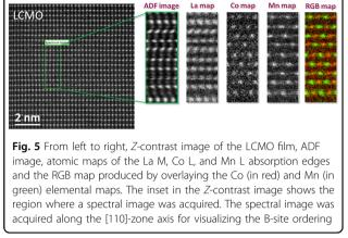
RGB map unambiguously demonstrates the Co/Mn ordering of the LCMO phase. Therefore, STEM images provide powerful confirmation that PAD growth promotes the desired double perovskite cationic ordering, as inferred from the optimal values of the *Msat* and Curie temperature.
