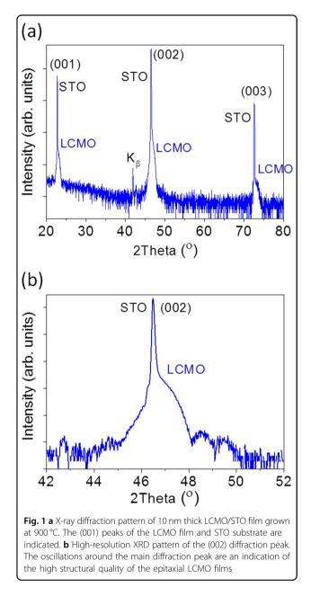
films grow epitaxially, cube-on-cube and fully strained with the STO substrate (Supporting Information, Fig. S3).
