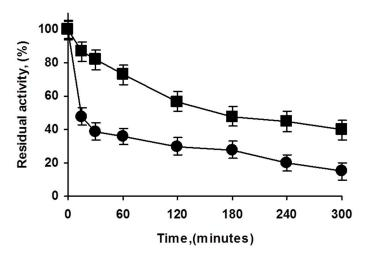
**Figure 3.** Effect of enzyme loading in the inactivation courses of octyl PFL biocatalysts. Inactivation carried out in 50 mM Tris at pH 7 and 75 °C. Experiments details as described in Methods. Squares: highly loaded biocatalyst; circles: lowly loaded biocatalyst.
