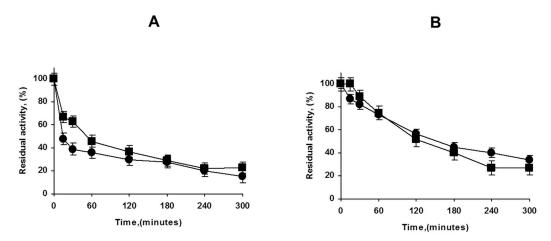
**Figure 4.** Effect of PEI coating of lowly (**A**) and highly (**B**) loaded PFL octyl biocatalysts. Inactivation carried out in 50 mM Tris at pH 7 and 75 °C. Other details are described in Methods section. Circles: unmodified preparations. Squares: PEI coated preparations.
