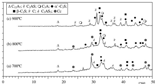
Figure 3. XRD diffractograms of FABC with calcinations temperature
