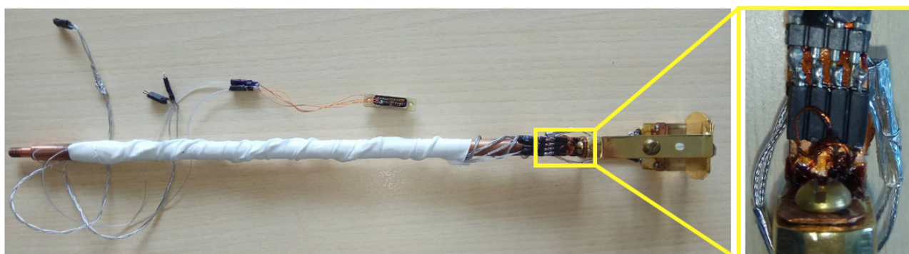
Figure 28. Left: insert of the dilution fridge. The far-right end part of the insert is the sample holder, where the sample is placed for the magnetic measurements. Right: close-up view of the thermometer.
