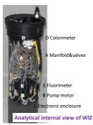
This multi-parameter system has been tested in several campaigns in automatic and continuous mode for more than 24 h, showing that it is a powerful tool for biogeochemistry studies in coastal areas.
