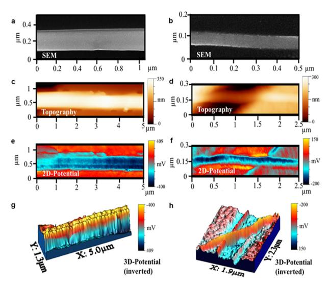
Figure 2. Surface potential ripples of  $Bi_2Te_3$  nanowires. SEM, (a,b), and AFM topography, (c,d), images of 250 nm and 45 nm diameter NWs. 2-dimensional, (e,f), and 3-dimensional, (g,h), KPM maps of the surface potential of the NWs.
