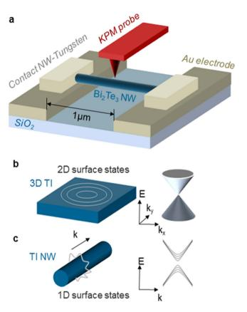
**Figure 1.** (a) Schematic diagram of the measurement set-up. (b) 3D topologoical insulators (TIs) exhibit 2D surface states, forming a Dirac cone. (c) TI nanowires exhibit 1D subbands on the surface, due to the quantum confined boundary condition along the perimeter direction.
