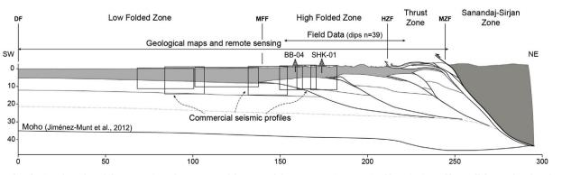
Fig. 5. Data distribution along the Erbil cross-section. The structure of the LFZ and the Outer HFZ is constrained by seismic profiles, well data and surface data, while the Inner HFZ and the Thrust Zone are exclusively based on surface data.
