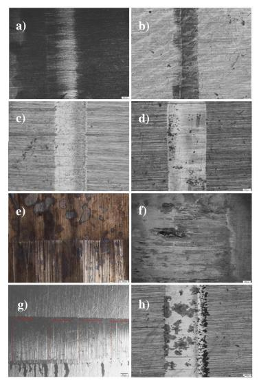
**Figure 2.** Optical microscope images (×500) of the wear scar in the blocks after tests with the different lubricating fluids: (a) PAO6, (b) PAO6 + graphene, (c) ChCl-urea, (d) ChCl-urea + graphene, (e) ChCl-malic ac., (f) ChCl-malic ac. + graphene, (g) ChCl-EG, (h) ChCl-EG + graphene.
