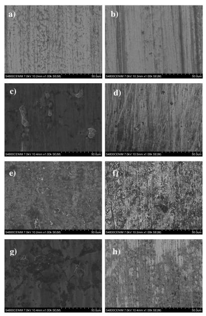
**Figure 3.** SEM images (×1000) of the wear scar in the blocks after tests with the different lubricating fluids: (**a**) PAO6, (**b**) PAO6 + graphene, (**c**) ChCl-urea, (**d**) ChCl-urea + graphene, (**e**) ChCl-malic ac., (**f**) ChCl-malic ac. + graphene, (**g**) ChCl-EG, (**h**) ChCl-EG + graphene.
