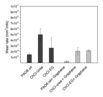
Figure 5. Average wear rate of the block (three tests) for each lubricating fluid.
