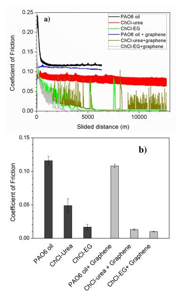
**Figure 4.** (a) Coefficient of friction recorder during the tests under different lubricating fluids, (b) Average coefficient of friction (three tests) for each lubricating fluid.
