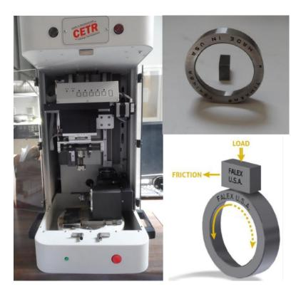
Figure 1. Tribometer and specimens used for the wear tests.
