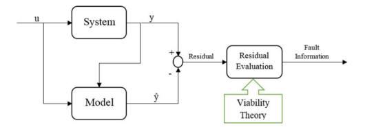
Figure 4. A general fault detection scheme.
