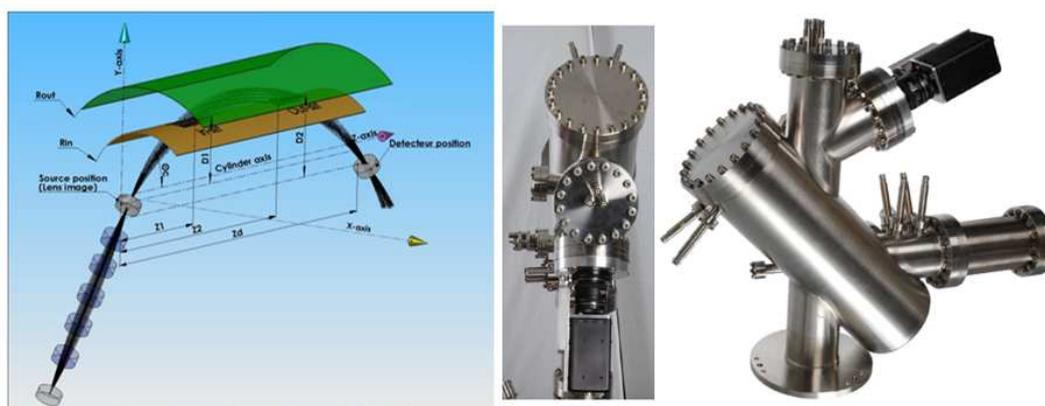
Figure 1. Schematic layout (left) of the HV-CSA dispersive analyzer. A pre-retarding lens system produces an image of the sample at the analyzer entrance slit. The voltage present between the two cylindrical plates deflects the electrons with the correct energy up to the exit slit and focuses on the electron detection system. (Right) Front and side pictures of the HV-CSA analyzer. The low dimension and weight enables its incorporation on a multipurpose experimental set-up.
