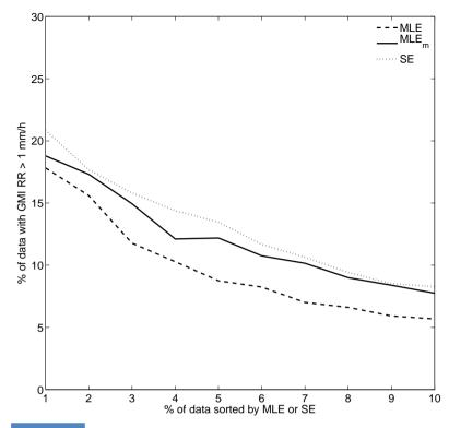
The probability of GMI RR> 1 mm/h as a function of the sorted percentiles by MLE (dashed curve),  $MLE_m$  (solid curve) and SE (dotted curve) (*a*) **outer swath** WVCs.
