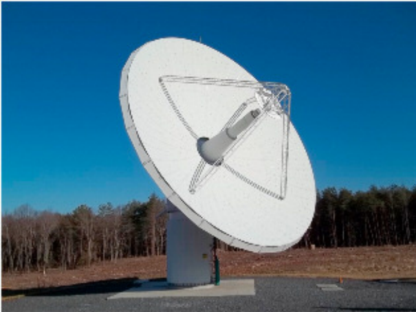
Figure 1. Photo of the 12-m-diameter VGOS antenna at the Goddard Geophysical and Astronomical Observatory site.
