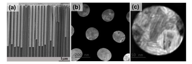
**Figure 1.** (a) Cross-section SEM image of AAO membrane filled with Co nanowires; (b) Top STEM image of the Co nanowires within the membrane; (c) closer look of a single nanowire presenting crystallites with different orientations.
