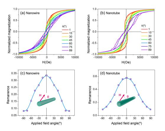
**Figure 4.** Simulated angular dependence of hysteresis loops for a single nanowire (**a**) and a single nanotube (**b**) and their respective remanence (**c**,**d**).
