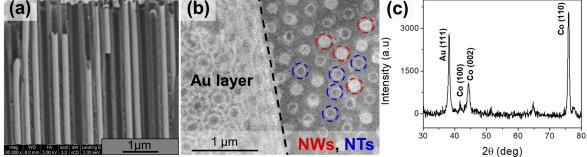
**Figure 2.** (a) Cross-section SEM image of AAO membrane filled with Co nanotubes; (b) top-view SEM image of nanotubes sample before and after a part of the Au layer was removed to image the nanostructures embedded into membrane; and (c) XRD pattern of the nanotubes within the AAO template whose peaks correspond to hcp Co phase and to the back sputtered Au layer.
