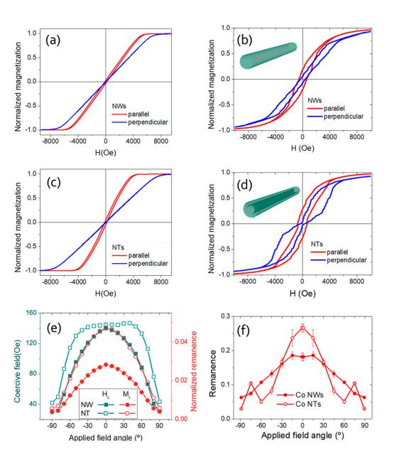
**Figure 3.** Experimental hysteresis loops for arrays of (**a**) nanowires and (**c**) nanotubes, respectively. Micromagnetic modelled loops of the arrays modelled in individual nanowire (**b**) and nanotube (**d**) with an effective 'interaction' anisotropy; (**e**) angular dependence of experimental coercive field and normalized remanence for nanowire and nanotube arrays; and (**f**) angular dependence of simulated remanence for nanowire and nanotube.
