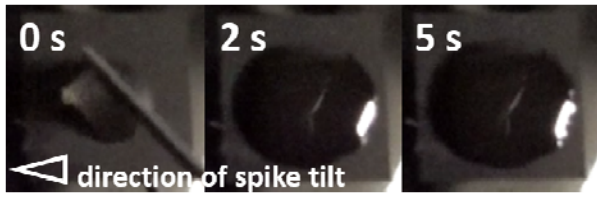
Fig. 8. Sequence of top-view photographs ( t = 0, 2 and 5 s after the oil droplet was placed on the surface) demonstrating the omnidirectional fluid transport of a droplet of engine oil ( 8 \mu\text{l} , Shell Rimula), placed in the centre of a surface of fs-laser processed tilted spikes [compare Fig. 4(f); irradiation conditions: angle of incidence 40^\circ , scanning perpendicular to the tilting axis, \phi_0 = 0.13 \text{ J/cm}^2 , N_{\text{eff}_1\text{D}} \approx 3.3 \times 10^4 ; processed area: 5 \times 5 \text{ mm}^2 ] on 42CrMo4 steel.
