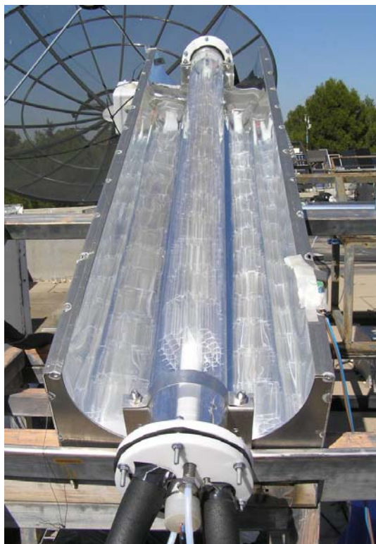
Figure 5. Photograph of the tubular photoreactor during operation with 14 photocatalytic PET monoliths at Ciemat.
