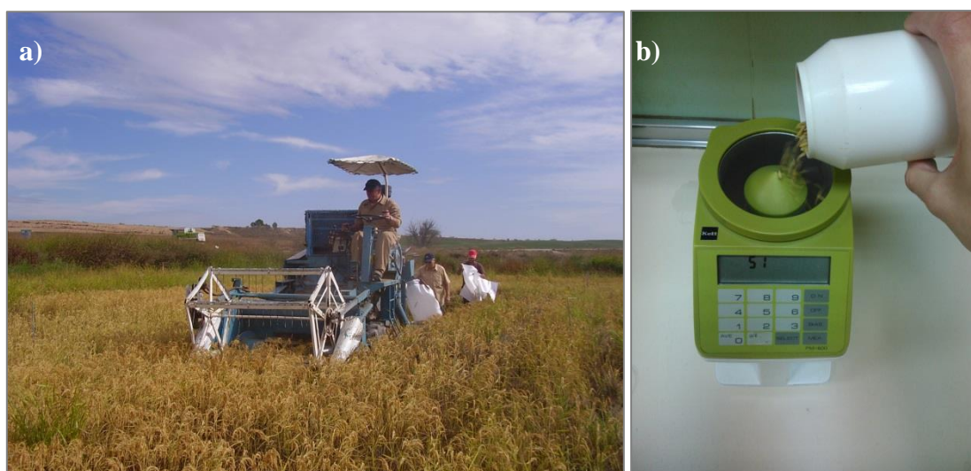
Figure 3.6. Villanueva de Sigena. Rice harvest with a commercial combine (a) and grain humidity measurement with the PM-600 grain moisture tester, Keller, Japan (b).
