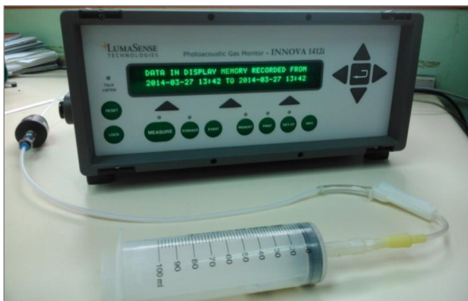
Figure 4.3. Innova 1412i Photoacoustic Multigas Monitor, used to quantify the gas concentrations.
