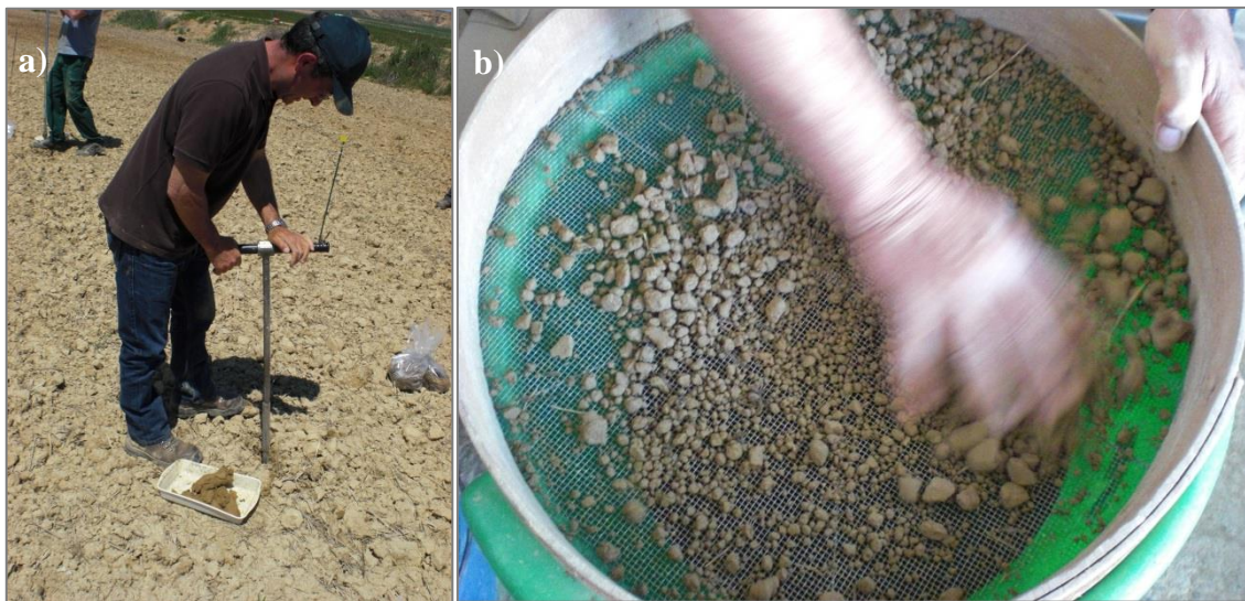
Figure 3.5. Villanueva de Sigena. Soil sampling before fertilization and seeding (a) and soil sieving (b).
