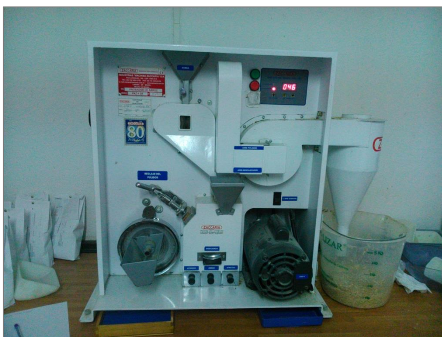
Figure 3.7. Milling process in a laboratory rice huller (PAZ-1-DTA, Zaccaria, Lineira, Brazil).
