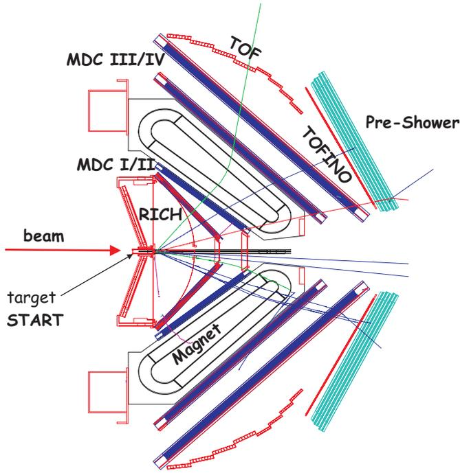
**Fig. 1.** Cut through two sectors of the HADES spectrometer. The magnet coils are projected onto the cut plane to visualize the toroidal magnetic field. The average distance between the target and the outermost detectors is about 210 cm.
