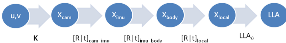
Fig. 41 Concatenation of coordinates transformation to georeference the victim
