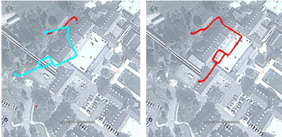
Fig. 22 Results (left) no integration of GPS with SLAM solution; (right) integration of GPS with SLAM solution [51]
