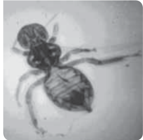
Figure 2. Radiography of a bee made with our source.
