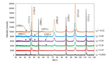
**Figure 2.** X-ray diffractograms for the initial microstructure (IM) and interrupted tensile-tested specimens at strains ( $\varepsilon_E$ ) of 0.10, 0.20, 0.30, 0.40, and fracture ( $\varepsilon_E$  = 0.52). Diamond dots indicate the presence of peaks associated to  $\varepsilon$ -martensite phase.
