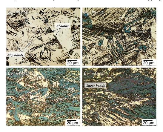
**Figure 3.** Light-optical micrographs of tensile-tested specimens interrupted at strains ( $\varepsilon_E$ ) of 0.10, 0.20, 0.30, and 0.40 after etching with Beraha's reagent for 10 s. The martensite phase is revealed in black and blue, whereas the austenite phase remains unetched.
