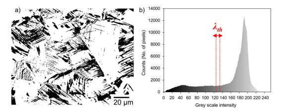
**Figure 4.** (a) Black-and-white image obtained from the light-optical micrograph of the condition strained up to  $\varepsilon_E = 0.10$  after applying a grey scale threshold value  $\lambda_{th} = 127$ ; (b) Histogram of the same micrograph showing the number of pixels vs. the grey scale intensity value.
