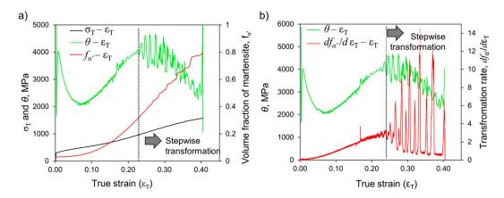
**Figure 10.** (a) Evolution of true stress  $(\sigma_T)$ , instantaneous work-hardening rate  $(\theta)$  and  $f_{\alpha \ell}$  with true strain  $(\varepsilon_T)$ . (b) Evolution of  $\theta$  and martensite formation rate  $(df_{\alpha \ell}/d\varepsilon_T)$  with  $\varepsilon_T$ . The dotted line highlights the origin of the stepwise transformation.
