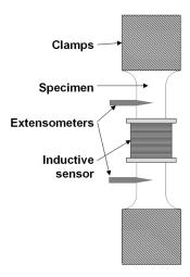
Figure 1. Tensile test setup with inductive sensor.
