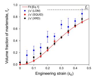
**Figure 5.** Evolution of martensite volume fraction ( $f_{\alpha \prime}$ ) with strain ( $\epsilon_E$ ) obtained ex-situ from interrupted tensile tests determined by LOM, magnetization measurements (SQUID), and XRD. The dashed line represents the saturation value of transformed martensite ( $f_s$  = 0.92) found by XRD for a sample strained to fracture.
