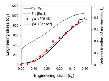
**Figure 8.** Engineering stress–strain ( $\sigma_E - \varepsilon_E$ ) curve and evolution of the  $\alpha'$ -martensite volume fraction ( $f_{\alpha'}$ ) with  $\varepsilon_E$  obtained by ex-situ magnetization measurements (SQUID), in-situ inductive measurements (sensor) and as predicted by the kinetics model.
