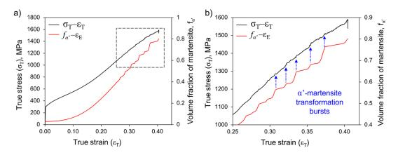
**Figure 9.** (a) True stress–strain  $(\sigma_T - \varepsilon_T)$  curve and evolution of  $f_{\alpha \prime}$  with  $\varepsilon_T$  obtained in-situ by using the sensor. (b) Magnification of the region marked with a square in (a) pointing out the effect of the transformation bursts on the strengthening of the material.
