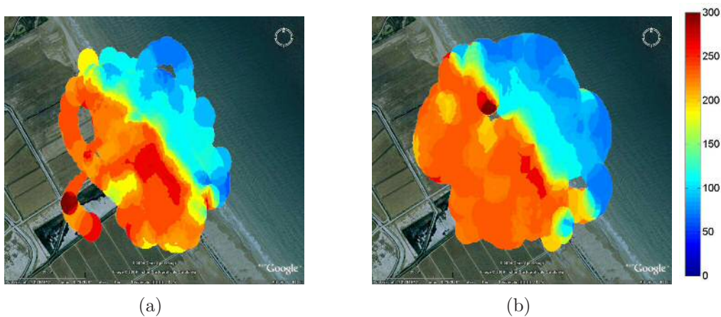
Figure 5.8 ARIEL Retrieved T_B [K] geo-referenced on Google Earth obtained at heights (a) between 40 and 170 m, and (b) between 170 and 300 m.
