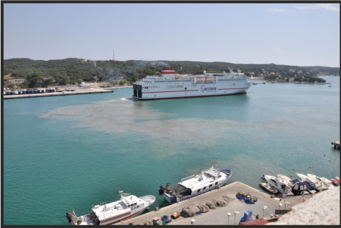
611 Fig. S2 A deep-draft vessel manoeuvring in the inner basin of Maó Harbour, and 612 resuspending sediments.
