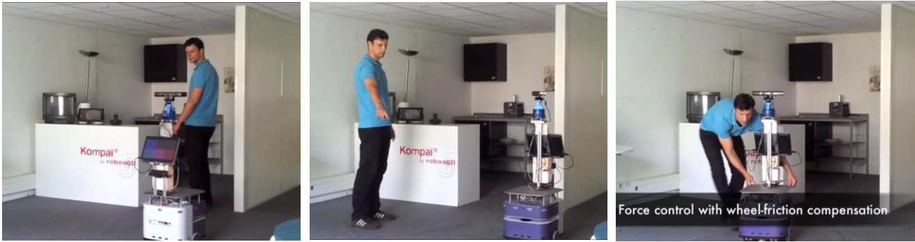
Fig. 4. Screenshots of three interaction modalities: person following (left); pointing control (center); direct physical interaction (right).
