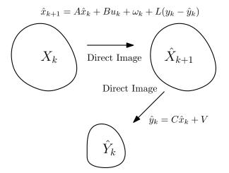
Fig. 1: Iterative algorithm of interval observer approach
