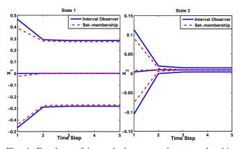
Fig. 4: Envelope of interval observer and set membership state estimation if 0 < LC < A
