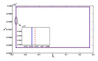
Fig. 7: The zonotope of state estimation in last iteration by both approaches for L = 0 (solid-line shows the interval observer and dashed-line presents the set-membership state estimations)
