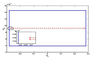
Fig. 5: The zonotope of state estimation in the last iteration by both approaches for 0 < LC < A (solid-line shows the interval observer and dashed-line presents the set-membership state estimations)
