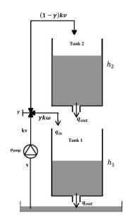
Fig. 3: Schematic diagram of the Two-tanks system
