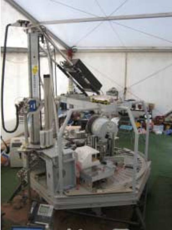
**Figure 17: DCSM with mounted equipment. The DCSM consists of a 3 legged fixed base, with rotating upper structure and vibration isolation deck.**
