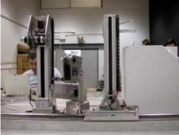
**Figure 9: CSHS Mechanisms for subsample acquisition and preparation. The systems are left to right: Sub-sampler, Crusher, SampleTransfer Mechanism.**
