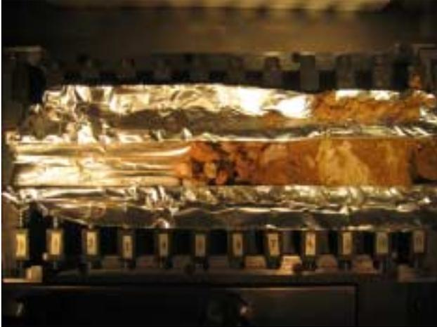
**Figure 10: Image of Core 24 from the Core Context Imager.** This camera provides an overall view of the core. Locations along the core are identified by the numbered labels.
