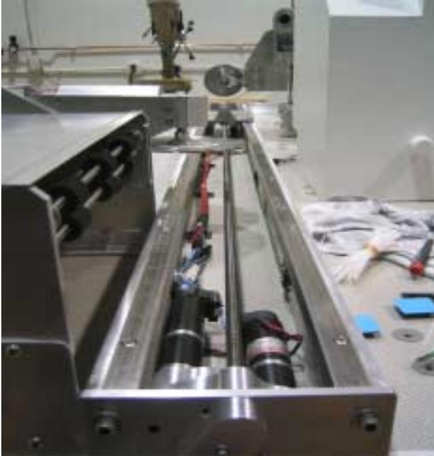
**Figure 6: CSHS Linear Rail.** The linear rail transports the clamp and core beneath instruments and the facing and subsampling saws.
