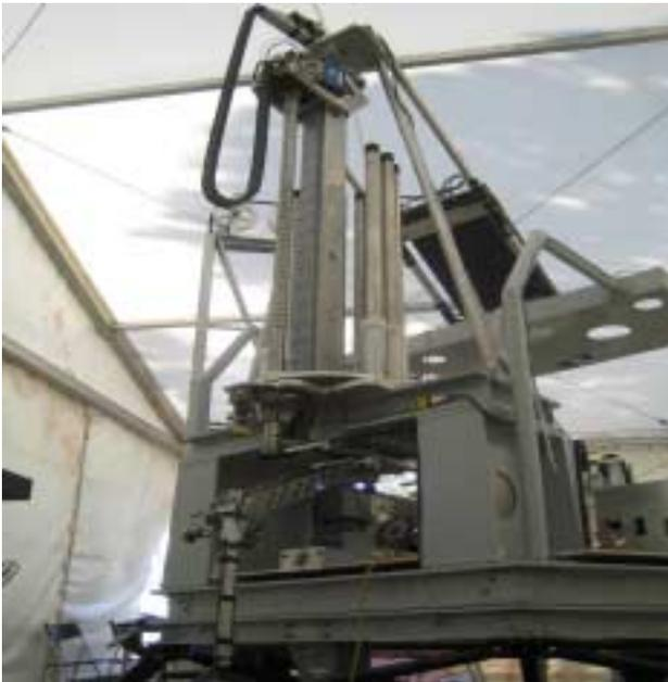
**Figure 3: The Drill Subsystem with lead drill string and coring bit attached. The drill system also includes a rotating cache with additional drill strings, and a Drill Core Hand-Off Mechanism.**
