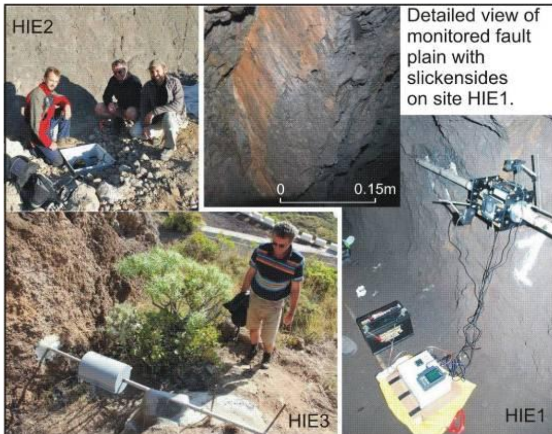
Fig. 2 Location and device characteristics of the monitored sites with the TM-71 crack gauge on the island of El Hierro. Photograph of the HIE1 shows the setting of the automated reading device installed on the TM-71 crack gauge. It consists of computer (white box on the floor), web cameras (on the crack gauge) and environmental monitoring station (dark box with large display on the PC, measuring air temperature/pressure and humidity). Electricity is supplied by car battery.
